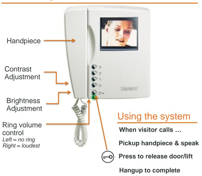
NOTE: Buttons labeled 0 to 3 are special function only, and not used in this installation.
